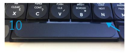
Now hinge the spacebar back over to the correct orientation, press down gently and the rear edge and push it back so it sits slightly under the first row of keys. See image. You can now press this down at the rear edge of the space and then slide it forward towards the front of the keyboard. By doing so, this engages the hooks on the rear of the spacebar with the pegs on the mechanisms.
