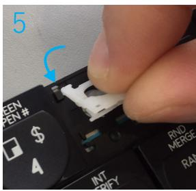
Slide the rear edge pegs into the slot on the keyboard tray. They should easily just slide in. You can then lower the front edge of the mechanism
