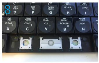
Please refer to the earlier steps 1-6 on how to remove the 1x1 keycap and install the new white mechanisms. The process is much the same albeit with a longer key. The space bar would still need to be lifted from the front edge to remove it, please be careful to lever it evenly. Note. You should now have a keyboard that looks like the image.
