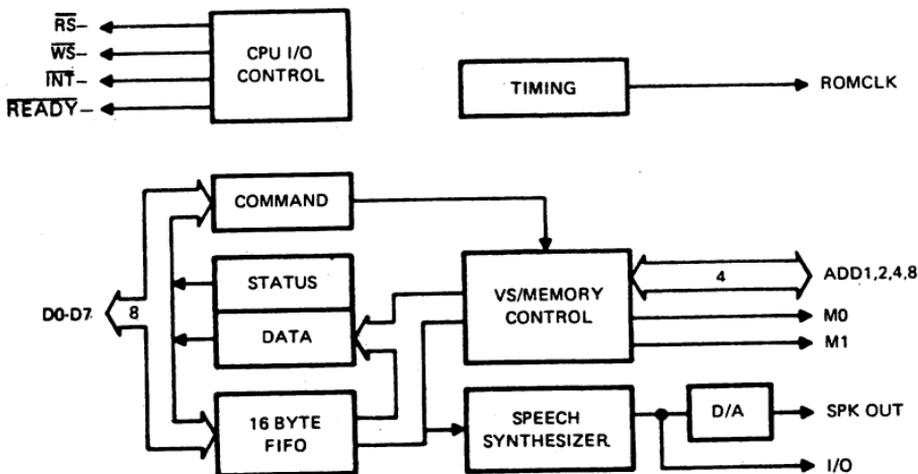
FIGURE 1 - VOICE SYNTHESIS PROCESSOR BLOCK DIAGRAM
