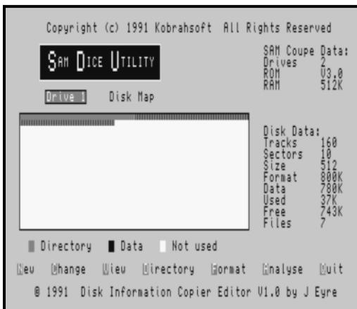
This display provides details about the number of tracks and sectors, sector size and the total disk format capacity available. If the disk is recognised as SAM format the number of current files, the amount of disk space allocated to current files and the space available for use is also identified together with a graphic indication of disk space used.
