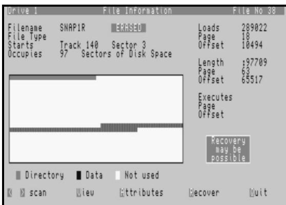
This display shows the filename followed by any file attributes or in the case of an erased file an erased indicator. Details of the location of the file and the amount of disk space used are displayed together with a disk map for the file.
