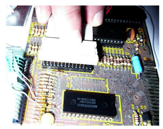
The result may look like this (the picture shows a demo board, the luster terminals are not necessary, the reset switch is just a cable which can be manually connected with GND i.e. with the modulator shield):
