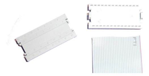
Shift the ribbon cable over the socket. The cable should fit tightly on the left and on the right side.
