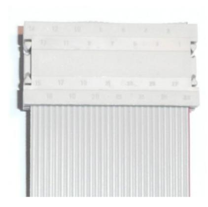
Use a pipe wrench or a similar tool to press the top and bottom of the socket together. First on the left hand side than on the right side followed by the middle (not shown here).
