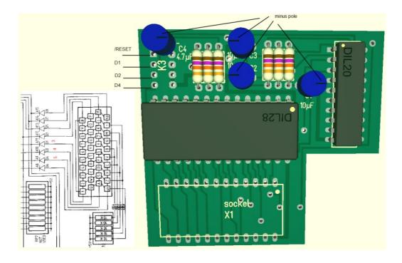
• Pull out the original ROM and plug in the MULTIROM connector.
