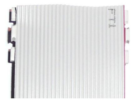
Put the upper part of the ribbon cable socket on top. The upper part must snap in.
