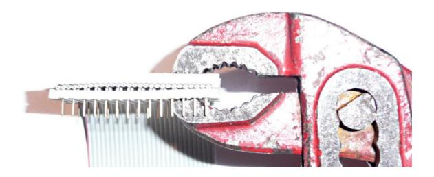
Install the socket on both ends of the cable to get the following:
