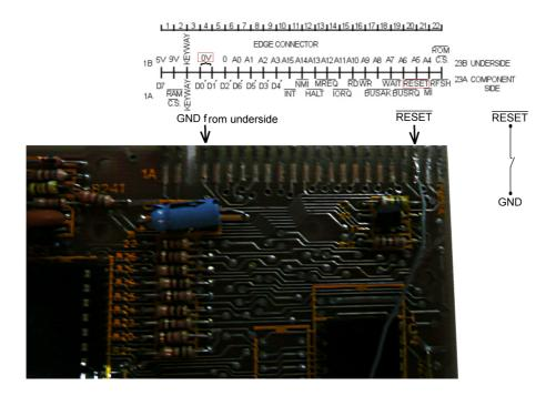
• Solder a cable to connect the signals D1, D2 and D4 from the ZX81 board with the multirom.
