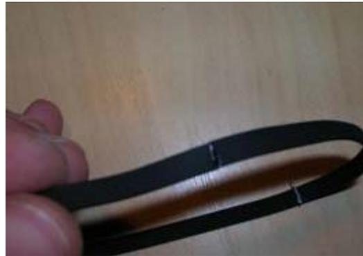
Reconnect the belt using the glue, don't exaggerate: a small quantity is enough. Spread the glue on the belt's cut using one needle. Important: Try to be sharp when joining together the two belt's parts; it's fundamental in the correct belt's spinning .
