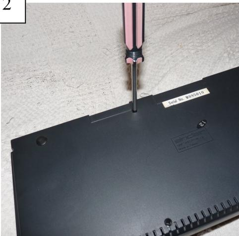
Be cautious when undoing screws as sudden torque can damage the plastic housing.
