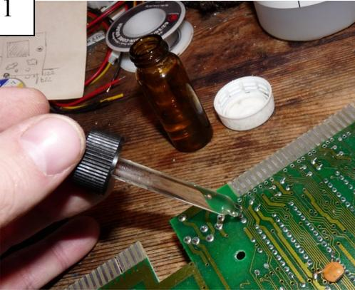
*Using No Clean – Non Corrosive Flux*
