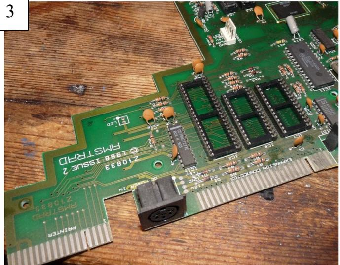
*Both ROM chips and Z80 CPU Removed*
