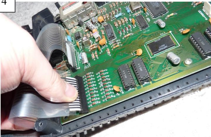
When removing the keyboard membrane tails from the connector, you should only need to use finger pinch pressure.
