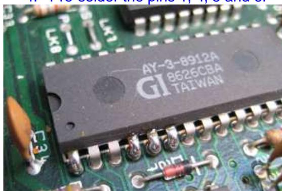
Pin 1 is the first pin anti-clockwise from the notch.
