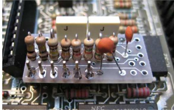
8. Solder the 2 wires to the ULA / matrix array:
