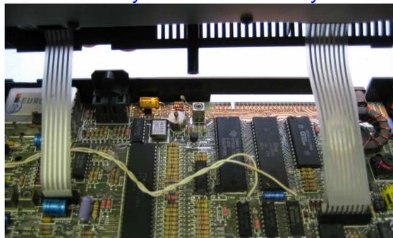
Also disconnect the taperecorder cable on the +2 / +2A / +2B.
