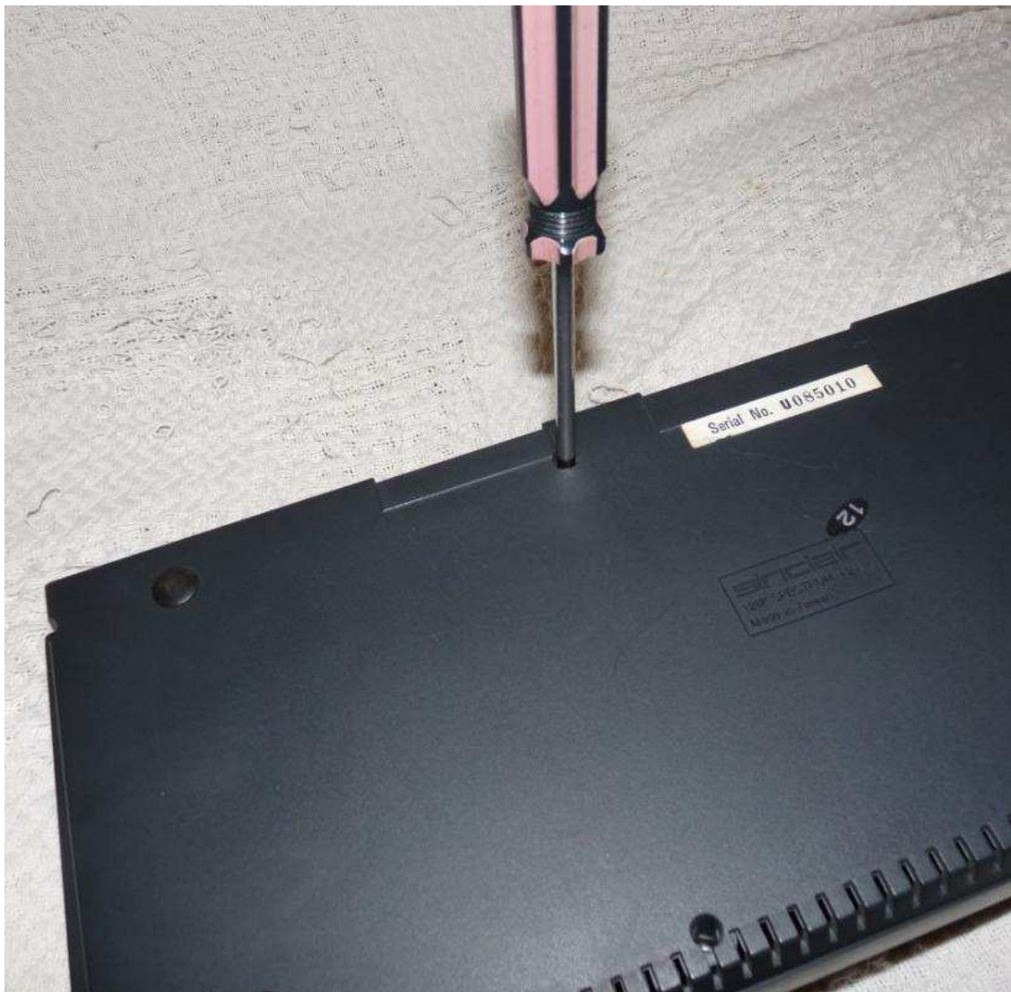
Gently does it, or you could break the plastic screw holders
