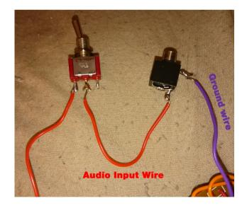
Drill two 6mm holes in the back of the +2 case and thread the switch and the audio socket through and reseat the datasette mechanism.
