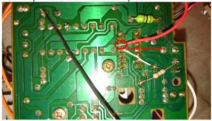
Next you need to locate a good place for the Ground wire. I found an empty hole on the PCB marked as 307 on the front of the PCB. This should give you a good place to solder the wire in.
