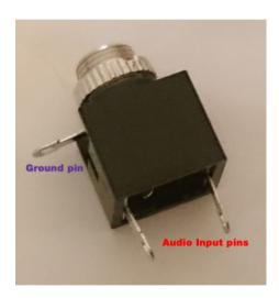
The audio input pins need to be wired together. You can either thread the audio in wire through the holes and then solder the wire to the pins or do what I do.
