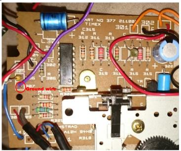
Next you need to connect the ground wire to the 3.5mm Socket
