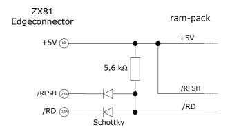
With this modification the refresh-signal to the ram-pack will be always high or disabled. The read-signal to the ram-pack is now activ low either if the CPU generated a read or a refresh. This makes the ram-pack send the memory data to the bus when a refresh cycle happens. For normal operation of the computer or the ram-pack this is regardles. The hrg-software on the other hand just needs these data to generate a graphic-video.
