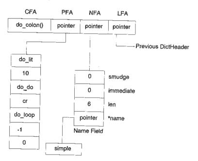
The run time function called by '(' is do\_do(). It pushes the number of times to loop and a zero for the index onto the return stack. The run-time function called by ')' is do\_loop(). do\_loop() calls branch() to jump to the top of the loop. Each time do\_loop() executes, the loop index on the Return Stack is incremented and tested to see whether to loop again or fall out of the loop.
