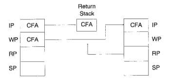
**EXIT** is the last macro executed at the end of a high level macro. It pops the CFA off the Return Stack into IP.
