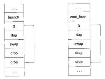
**LOOPING** CALL supports only one looping construct, (...). Other structured looping constructs, such as *begin* ... *until*, can be easily added to the compiler. Looping operators are restricted due to space limitations and to keep CALC simple for the user to learn.
