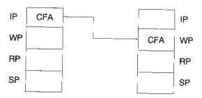
**EXECUTE** expects the CFA on the Parameter Stack. It loads the CFA into WP. The macro is then executed either with a jump (JMP) to WP or a subroutine call (JSR). EXECUTE is called RUN in some early TILs.
