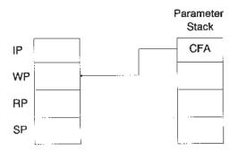
**DOCOLON** assumes that the CFA of the macro to return to is in the IP and the CFA of the current macro to execute is in WP. The CFA in WP is converted to a Parameter Field Address (PFA). The contents of the IP is pushed onto the Return Stack, modifying RP. The CFA contained in the PFA is moved into IP, then NEXT is invoked. DOCOLON is the primitive routine whose address is compiled into the CFA of a high level macro. DOCOLON is also named NEST in some older TILs.
