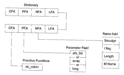
The PFA can be one of several data types. A C++ union is used to define the PFA. The following code defines a dictionary entry:
