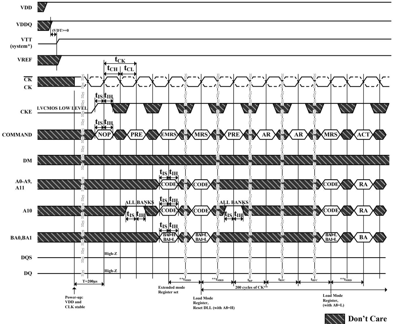
\*=VTT is not applied directly to the device, however  $t_{VTD}$  must be greater than or equal to zero to avoid device latch-up.
