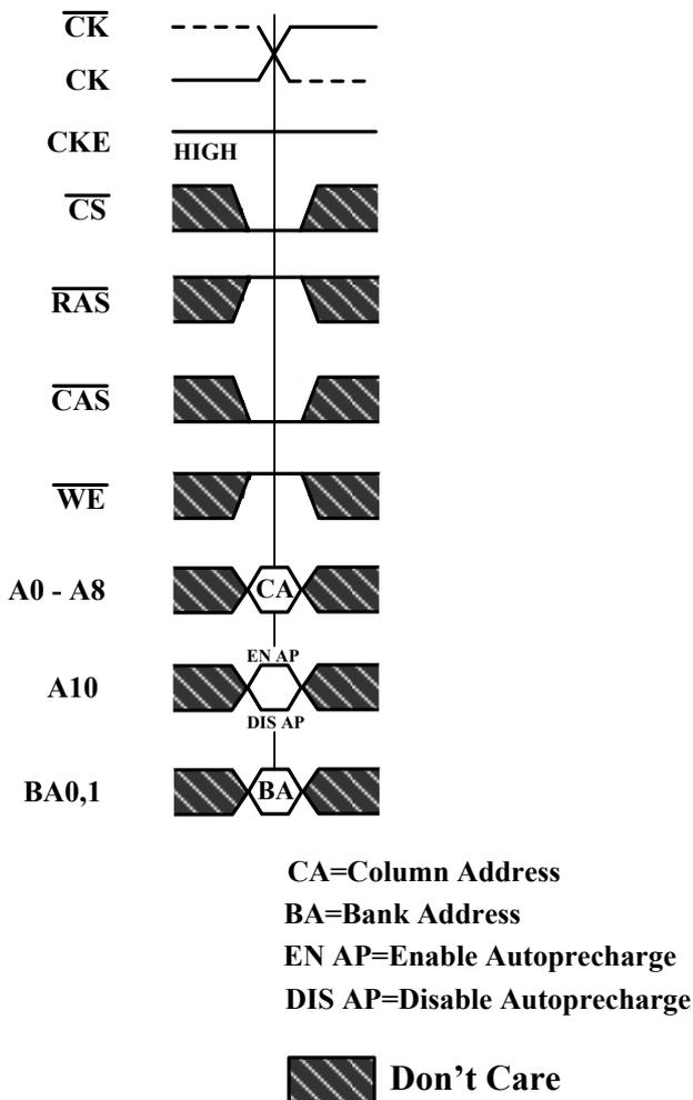
**Figure 8. Read Burst Required CAS Latencies (CL=2)**
