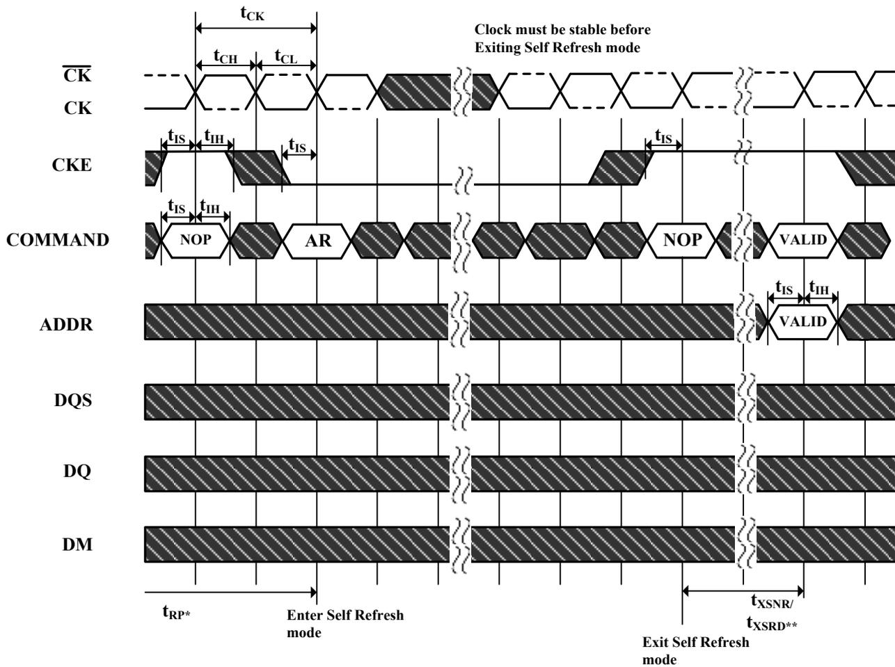
\* = Device must be in the "All banks idle" state prior to entering Self Refresh mode
