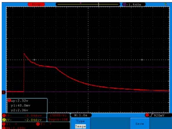
Figure 8: Initial configuration: ROMs and Zener Diode ZD5 installed. Voltage at ROM socket.
