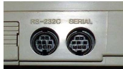
**Figure 2:** Left: Cable to connect the serial interface to a PC. Top: The Mini-DIN connector must have a small outer diameter to fit into the case.
